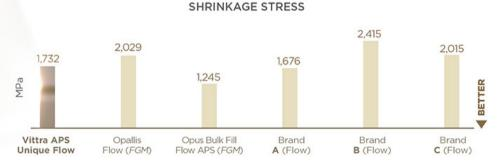
Vittra APS Unique Flow showed a result equivalent to the average performance of the main four competitors. The lower the contraction and tension generated, the lower the risk of marginal infiltration and greater the longevity of the restoration.
